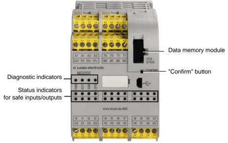
Figure 3-4 Operating and indication elements of the safety contoller
