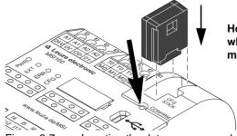
Hold down the "Confirm" button while inserting the data memory module
