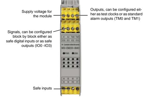
Figure 4-4 Signal connections MSI-EM200-8I4IO
