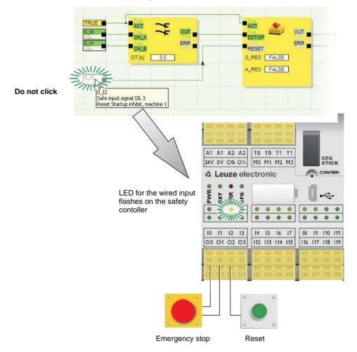
At the same time, the LED for the corresponding input/output flashes on the safety contoller or on the corresponding safe extension device.
