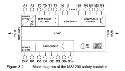
The safety contoller can be used both with and without extension modules.
