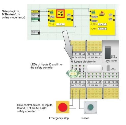
Therefore, the LEDs for inputs I0 and I1, which are both directly connected to this functional block, flash on the safety contoller.
