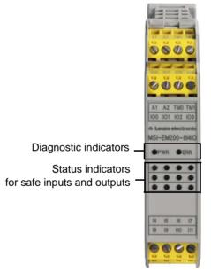
Figure 4-3 Diagnostic and status indicators on the extension device
