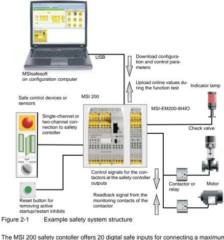
The diagram below illustrates the overall system in an application example.
