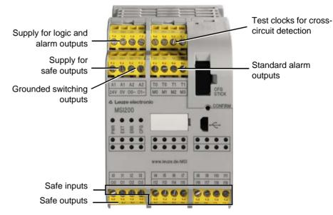
Figure 3-5 Signal connections MSI 200
