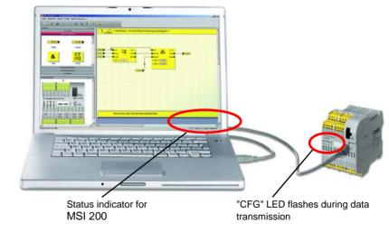
Figure 6-4 USB connection between PC and safety contoller
