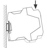
Figure 3-10 Snapping the MSI 200 safety contoller onto the DIN rail
