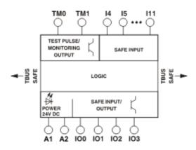
Figure 4-2 Block diagram MSI-EM200-8I4IO
